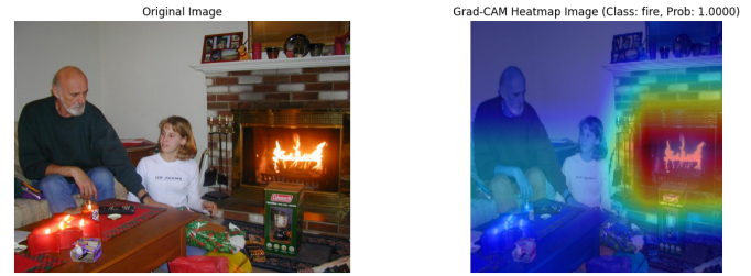
Fig. 13. Original image on the left. On the right, the image consists of the heat map of the Grad-CAM visualizing the feature (pixels) importance. Furthermore, the second image has the detection class with the Confidence Score.
